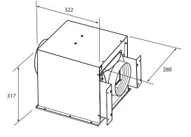
The twin fan motor assembly installs into the roof space above the kitchen. It simply plugs into a cable from the rangehood
